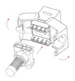
Insert the cable through the termination cap ensuring the cap fits just on the end of where the cable is stripped back to, untwist the four pairs and fan out. Following the colour code on the cap, insert the wires into their designated slots. Double check the wires are in the correct positions and then trim off the excess.
